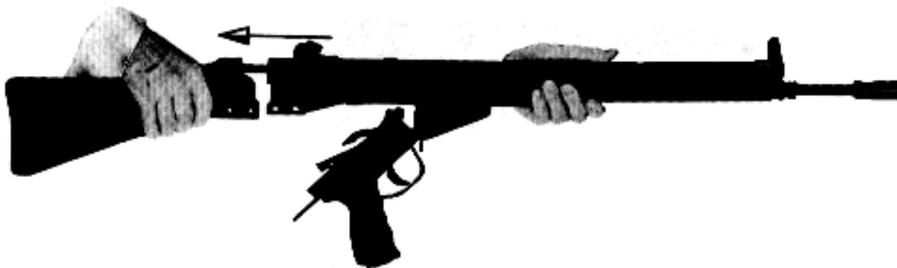
Fig. 63: Remove back plate with butt stock
