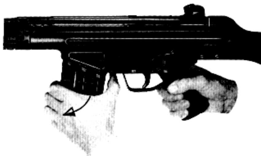
Fig. 54: Removal of magazine
