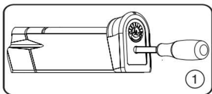
A) Use a **punch** to press in on **magazine spring seat/clip**.
