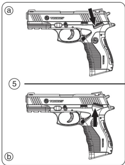
5. If you want to stop shooting before firing the last cartridge of a magazine, decock the firearm immediately by moving the **safety** downward (a) and push the safety lever in the up (on) position (b).
