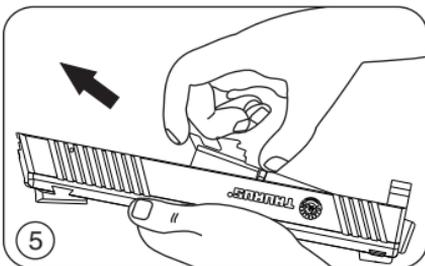
5. Remove the **barrel** from the **slide** by pulling to the front and up.
