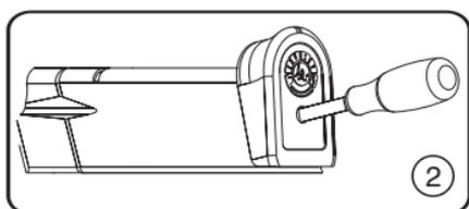
C) Withdraw **magazine spring plate** and **magazine spring** from **magazine body**. Turn magazine upside down and remove magazine follower.
