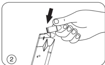
2. Hold the **magazine** with one of your hands and with the other one insert the cartridges one at a time, pressing them down and to the rear. Insert the **magazine** into the pistol until it is held by the **magazine catch**. If the **magazine** is not correctly inserted into the pistol, it can be dropped when you intend to shoot.
