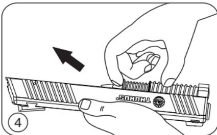
4. Release **slide spring assembly** from its position on the bottom of the **barrel**.
