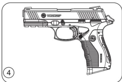
4. The pistol is now cocked and ready to fire by pulling the **trigger**. After firing, the **slide** will recoil from gas pressure and will eject the empty cartridge case and feed another cartridge into the chamber. The pistol will be ready to fire again. After the last round, the **slide** will remain in the open position held by the **slide catch**. In order to make it return to its rest position, press the **slide catch** just above the **left grip**.
