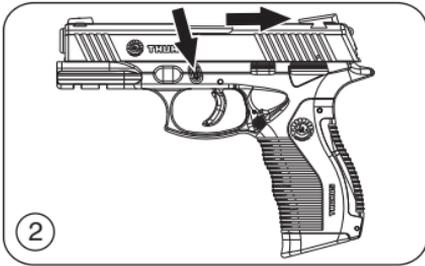
2. Hold the pistol according to figure and with four fingers, keep the **slide** in its backward position approx. 1/8". Simultaneously, with the other hand's thumb and index finger, pull the **disassembly latch** down. Push the slide to its forward position before releasing the disassembly latch.
