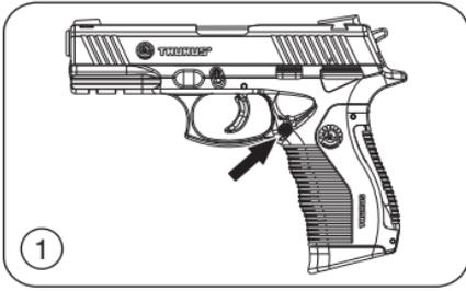
1. Remove the **magazine** by pressing the **magazine release button**.
