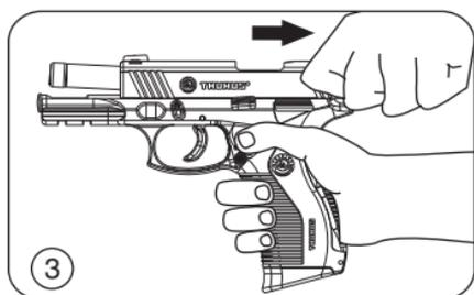
3. Hold the pistol with one hand keeping your finger away from the trigger. With the other hand pull the **slide** to its limit and release it, so slide will go forward under **recoil spring** pressure and will insert one cartridge in the chamber.
